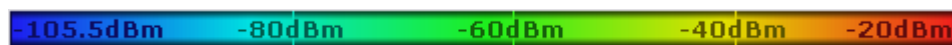
Fig. 3-49: Linear color curve shape = 0; colors are distributed evenly over the complete result range
