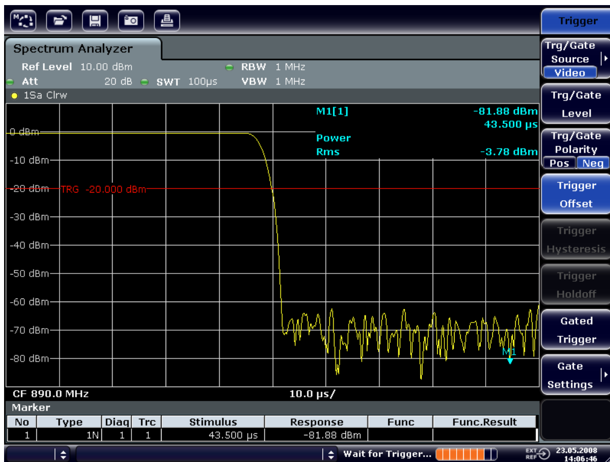
Fig. 2-20: Falling edge of the GSM burst displayed with high time resolution
